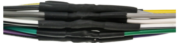
Soldering provides solid connections and a neat assembly with minimal bulk.
