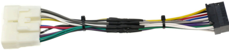
Soldering provides solid connections and a neat assembly with minimal bulk.
